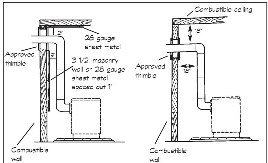
**Table 2: Clearances Using Clearance Reduction Systems**
